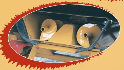
The two heavy-duty and high capacity augers mounted in the **belly pan**, convey the product to the discharge conveyor. The auger and pan combination provides for a high-speed transfer of the product and for a clean, leak-free environment under the tub grinder.
